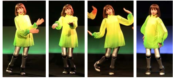
Fig.2 Dance demonstration performed by biped humanoid robot HRP-4C [7]. The motion of the robot was created using Choreonoid.
